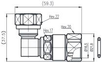
4.3-10 Right Angle male Connector for 1/2" Flexible RF Cable
